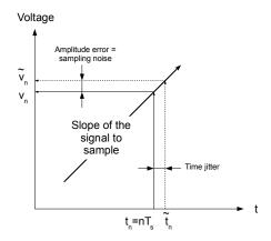
Figure 6: Time Jitter ⇒ Amplitude Error
