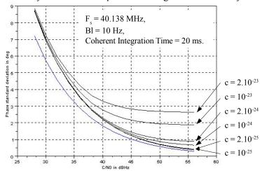
Figure 10: Phase Tracking Error Standard Deviation vs C/N0 and Constant c
