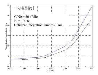
Figure 12: Phase Tracking Error Standard Deviation vs F<sub>s</sub> and Constant c
