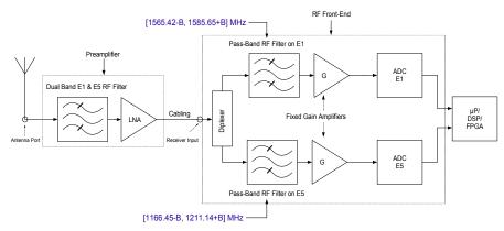
Figure 3: Direct Separate Sampling Architecture
