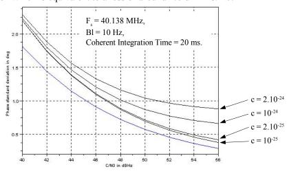
Figure 11: Phase Tracking Error Standard Deviation vs C/N0 and Constant c, a close-up view.
