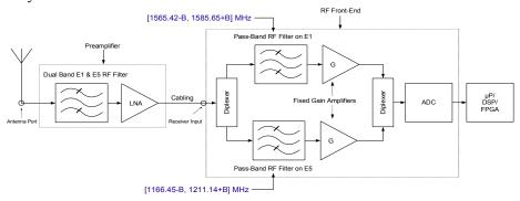
Figure 1: Direct Coherent Sampling Architecture
