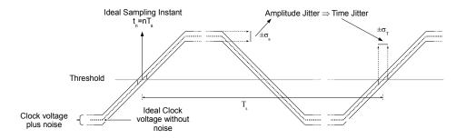
Figure 7: Aperture Jitter
