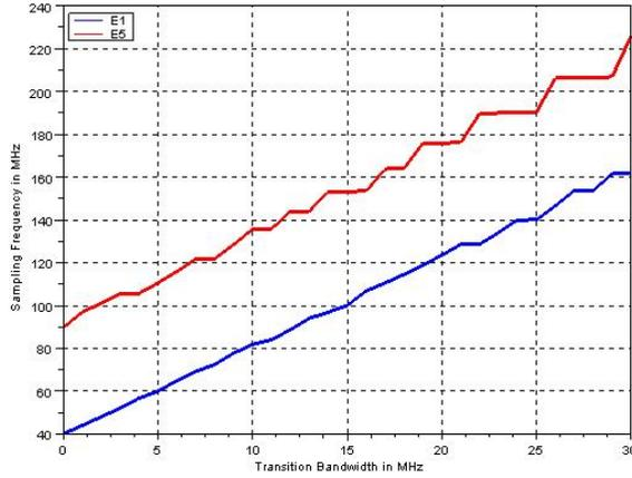
Figure 4: Minimum Sampling Frequency for Separate Sampling, as a function of the transition bandwidth
