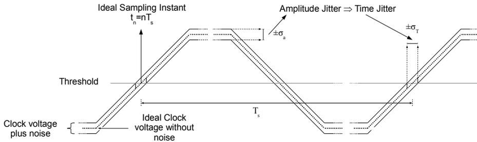
Figure 7: Aperture Jitter
