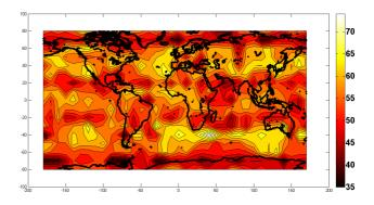
Figure 1- Smallest Critical Bias for APV 1 operations  $P_{f_{17,1}} = 2 \times 10^{-3}/h$
