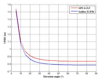
Fig 4– GPS L1/L5 and Galileo E1/E5b smoothed ionofree UERE
