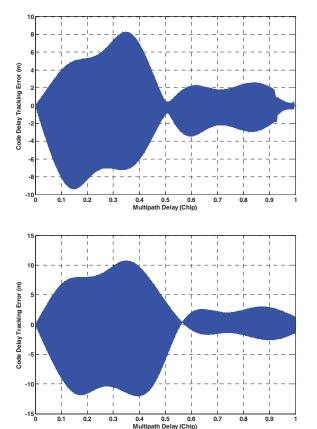
Figure 10 – DET and ASPeCT Code Delay Tracking Error in Presence of Multipath (half the Amplitude of the Direct Signal).
