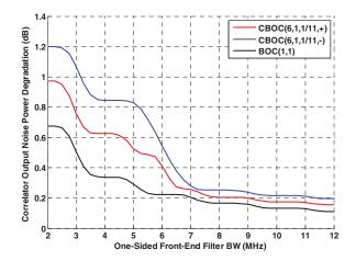
Figure 1 – Correlator Ouput Noise Power Degradation According to the Local Replica.
