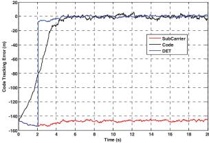
Figure 8 – DET Code Delay Tracking Error for an Initial Error of 0.5 Chip and a C/No of 45 dB-Hz (Top) and 30 dB-Hz
