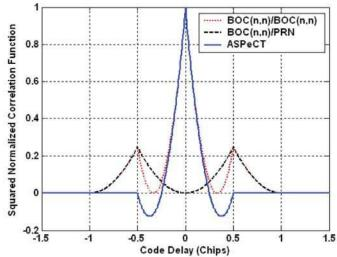
Figure 2 –BOC(1,1)/ BOC(1,1), BOC(1,1)/PRN Squared Normalized Correlation Functions and ASPeCT Modified Correlation Function Without Front-End Filter
