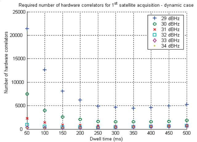
Figure 15 Required number of hardware correlators vs dwell time for the first satellite acquisition – dynamic case
