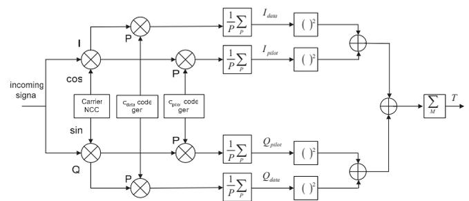
Figure 1 Acquisition process structure
