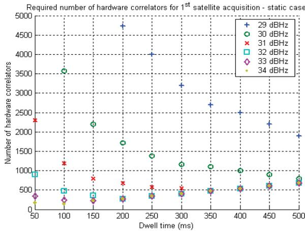
Figure 17 Close-up - required number of hardware correlators vs dwell time for the first satellite acquisition – static case
