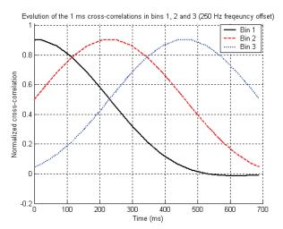
Figure 9 Evolution of 1 ms cross-correlations computed in bins 1, 2 and 3 for a frequency offset of 250 Hz
