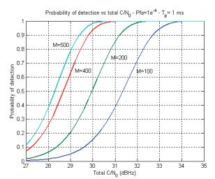
Figure 3 Probability of detection as a function of the total  $C/N_0$  for several numbers of non-coherent integration – 1 ms coherent integration
