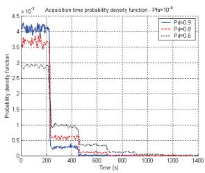
Figure 6 Acquisition time probability density function for Pd=0.9, 0.8 and 0.6
