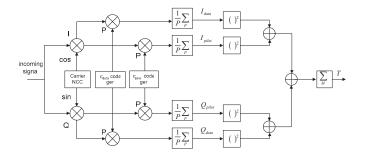
Figure 1 Acquisition process structure
