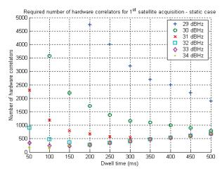
Figure 17 Close-up - required number of hardware correlators vs dwell time for the first satellite acquisition – static
