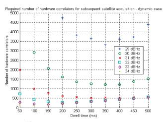
Figure 18 Close-up - required number of hardware correlators vs dwell time for subsequent satellite acquisition – dynamic case
