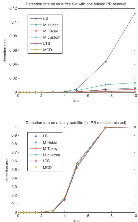
**Figure 9: False alarm and true fault detection rates**
