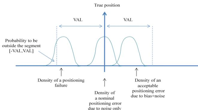
**Figure 3 - Vertical positioning failure**
