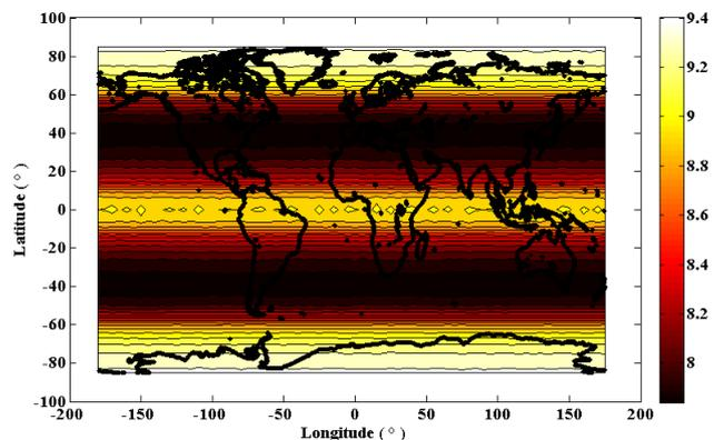
**Figure 6 - Average number of satellites over 1 day considering 27 satellites Galileo constellation (mask angle 10°)**
