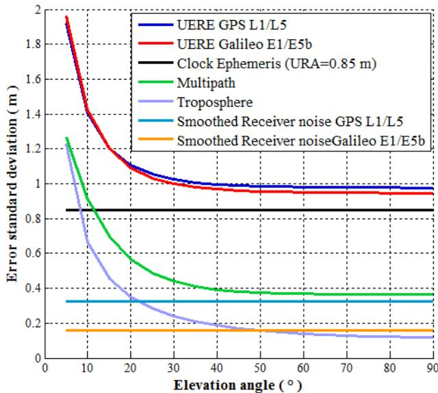
Figure 1 – User equivalent range error components
