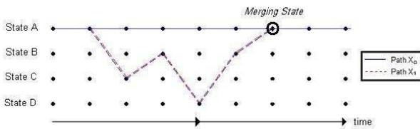
Figure 6: Viterbi Trellis - Two sequences merging at a State
