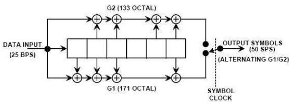
Figure 4: Encoding of the GPS L2C/L5 convolutional code (171,133)
