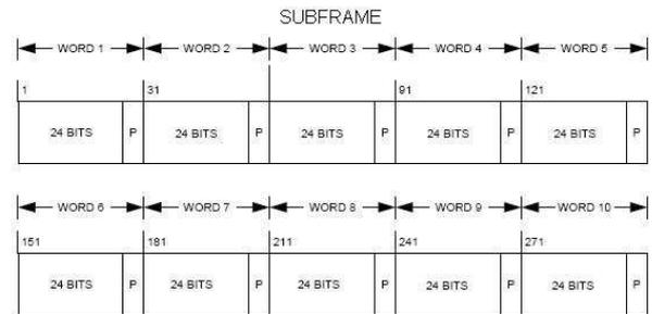
Figure 2: Subframe of the GPS L2C mode NAV data navigation message
