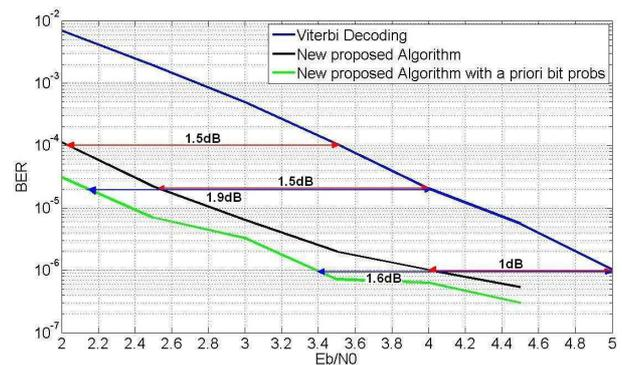
Figure 13: GPS L2C mode NAV data Decoding Performance: BER vs  $E_b/N_0$  for the Viterbi Algorithm, the New Proposed Algorithm and the New Proposed Algorithm with a priori bit probabilities - 4000 candidates
