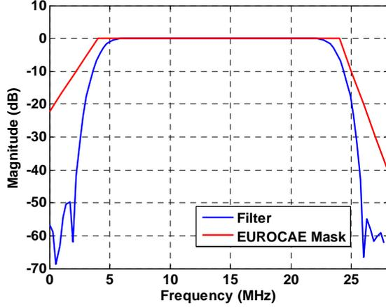
Figure 7: Simulator FIR Transfer Function Magnitude.
