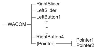
Figure 6. Internal structure of a Wacom device
