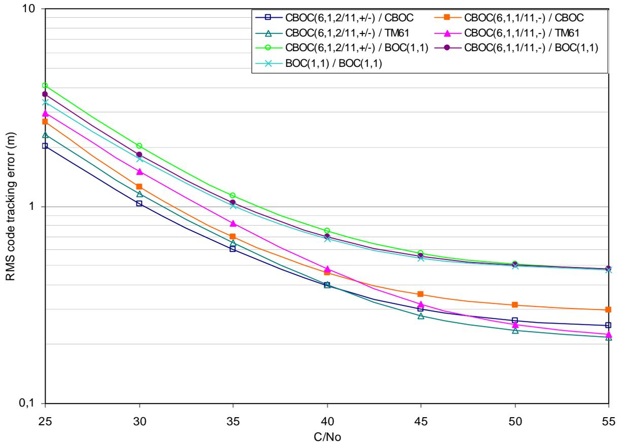
**Fig 7: RMS code tracking error in meter for BOC(1,1) signal and CBOC signal received by a CBOC receiver, a TM61 receiver a BOC(1,1) receiver, front-end filter bandwidth 8MHz one sided, urban multipath environment**
