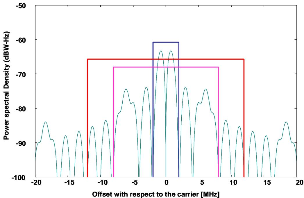
Fig. 4: Power spectral density of MBOC(6,1,1/11) and considered front-end filters bandwidths
