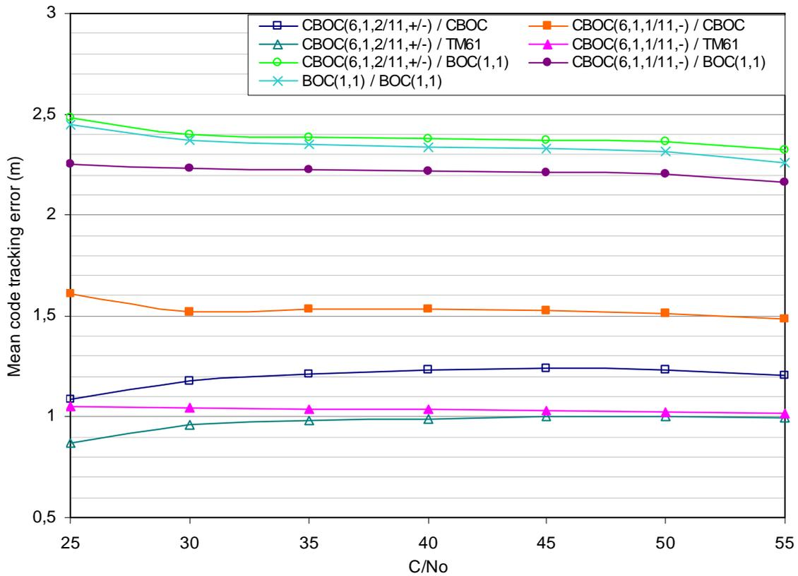
**Fig 8: Mean code tracking error in meter for BOC(1,1) signal and CBOC signal received by a CBOC receiver, a TM61 receiver a BOC(1,1) receiver, front-end filter bandwidth 8MHz one sided, in urban multipath environment**
