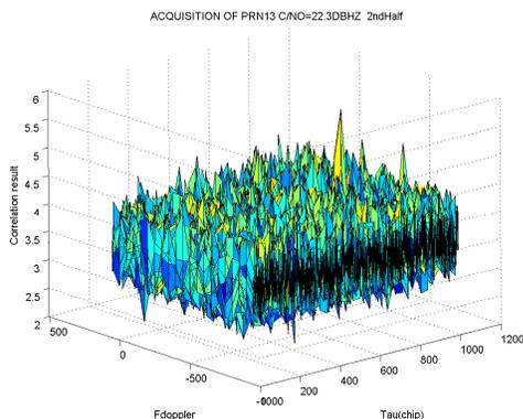
Figure 14: Acquisition matrix for the PRN13 set 2
