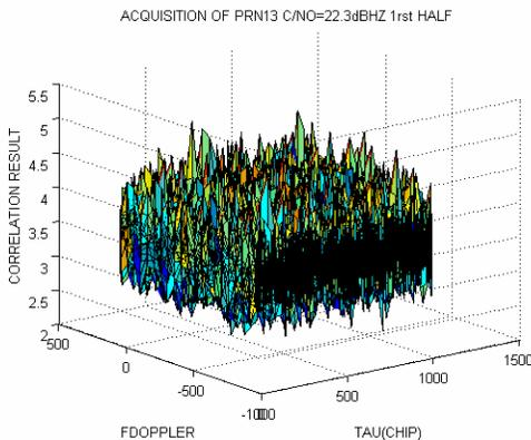
Figure 13: Acquisition matrix for the PRN13 set 1
