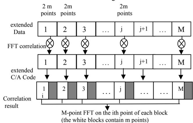
Figure 16: FFT Block correlation and FFT transformation
