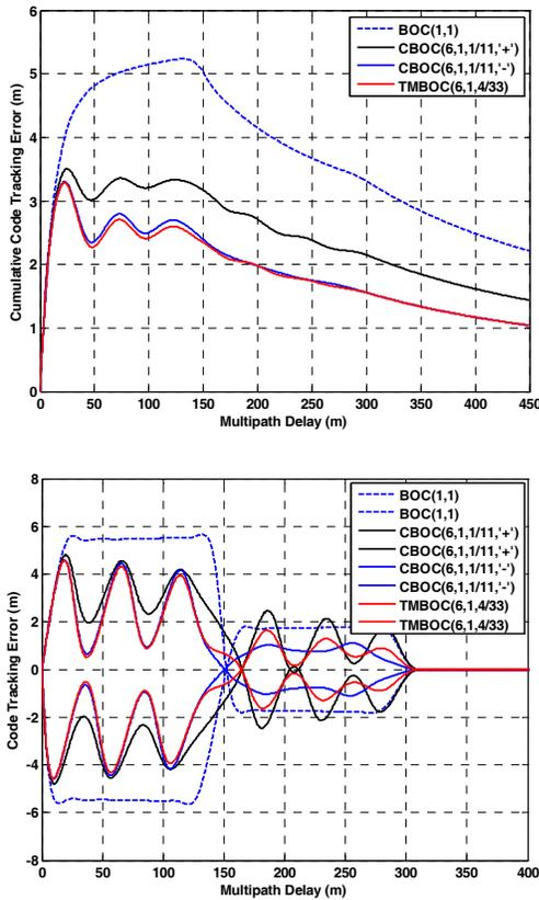
**Figure 3 – CBOC(6,1,1/11,-) and TMBOC(6,1,4/33) Running Average Multipath Errors (Top) and Multipath Envelope (Bottom) Assuming a 1/12 Chip Early-Late Spacing, and a 12 MHz One-Sided Filter, and a 3 dB SMAR**
