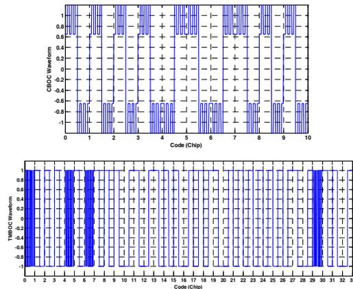
**Figure 1 – Truncated CBOC(6,1,1/11,'-') (Top) and TMBOC(6,1,4/33) Waveforms**
