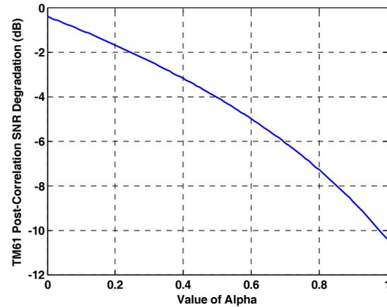
Figure 5 – TM61-Induced Post-Correlation SNR Degradation for CBOC(6,1,1/11) Signals
