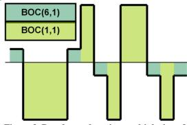
Figure 2. Pseudo-random time multiplexing of BOC(6,1) and BOC(1,1) in the CBOC solution
