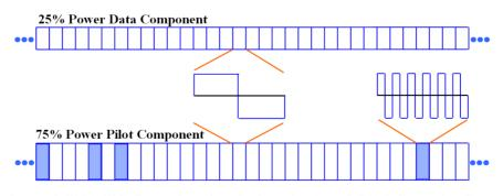
Figure 6. Example of TMBOC(6,1,4/33) Spreading Time Series, with All BOC(6,1) Spreading Symbols in the 75% Pilot Power Component
