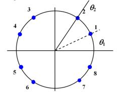
Figure 3. Modified Hexaphase modulation with constant envelope for the optimized signal
