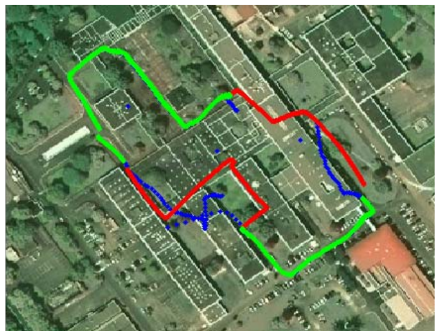
Figure 16 – AGPS/IMU Hybridization Results. Long Test with Corrected Regression Coefficients (Post Processing Results).
