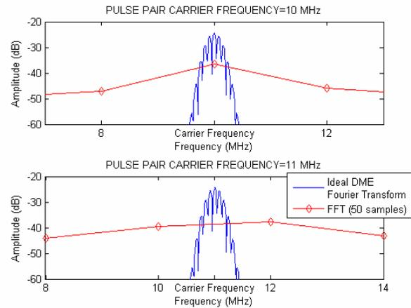
**Figure 5: FFT's Resolution and Distortion Issues ( $F_s=100$  MHz)**
