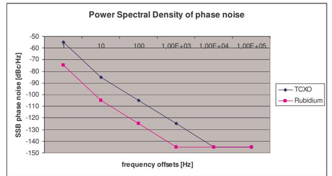
Figure 12: Power Spectral Density of TCXO and rubidium receiver clocks
