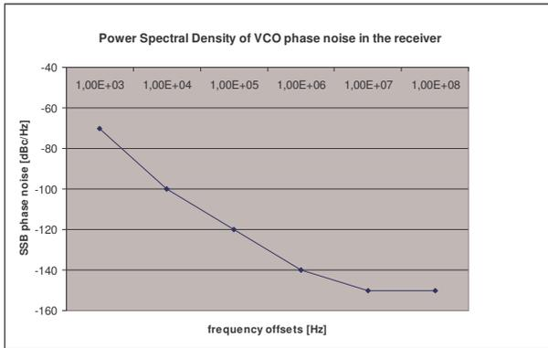
Figure 13: VCO phase noise power spectral density
