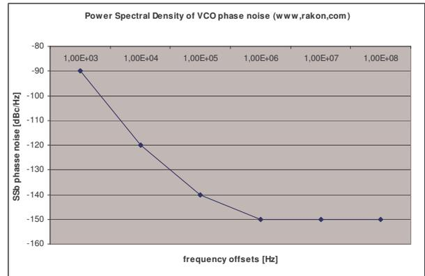
Figure 7: Power Spectral Density of VCO phase noise
