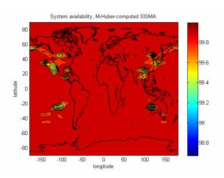
Figure 4: System availability over 24 hours, with M-Huber algorithm
