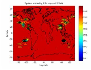
Figure 3: System availability over 24 hours, with LS algorithm
