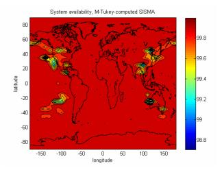
Figure 5: System availability over 24 hours, with M-Tukey algorithm
