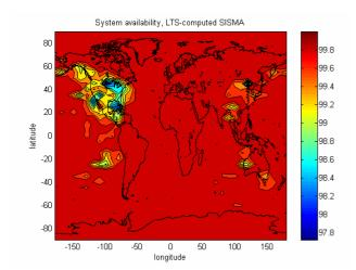
Figure 7: System availability over 24 hours, with LTS algorithm
