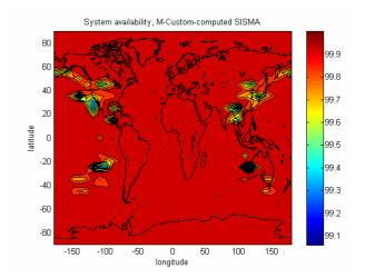
Figure 6: System availability over 24 hours, with M-custom algorithm
