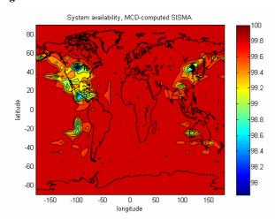
Figure 8: System availability over 24 hours, with MCD algorithm  $\,$
