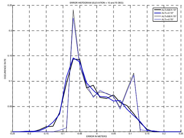
**Figure 18:** Observed distribution of smoothed code tracking errors for elevations 10° and 70° (GPS L1 C/A, BW<sub>2</sub>=2 MHz, C<sub>S</sub>=1 chip, ground reflection amplitude×2, 500 approaches per sat elevation, A340).
