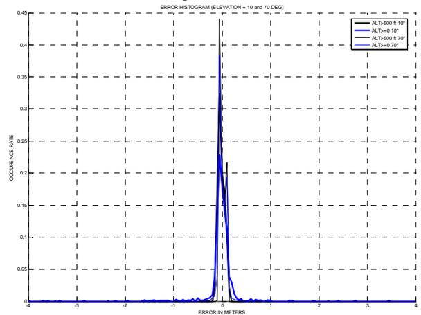
**Figure 19:** Unsmoothed code tracking error distribution at 10° and 70° (GPS L1 C/A, BW<sub>2</sub>=2 MHz, C<sub>S</sub>=1 chip, 500 approaches per sat elevation, A340).
