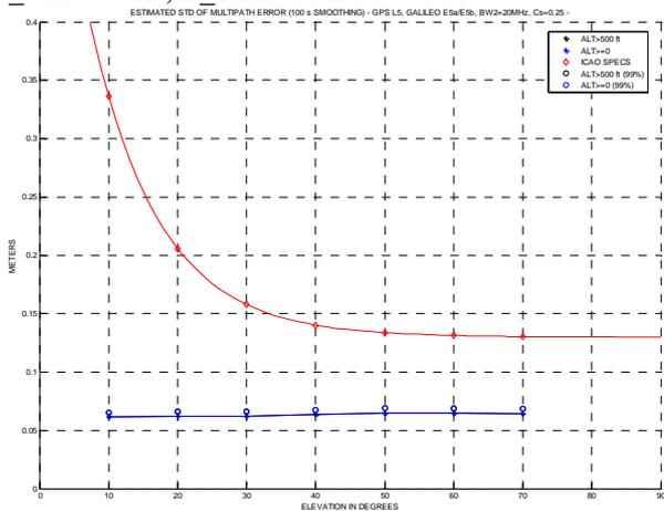
**Figure 25:** Smoothed pseudorange error sigma compared to SARPS model (GPS L5, GALILEO E5a/E5b,  $BW_2=20$  MHz,  $B_{PLL}=10$  Hz,  $B_{DLL}=1$  Hz,  $C_S=0.25$  chip, 500 approaches per sat elevation, A340).
