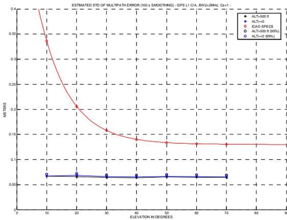
**Figure 16:** Smoothed pseudorange error sigma compared to SARPS model (GPS L1 C/A, BW<sub>2</sub>=2 MHz, C<sub>S</sub>=1 chip, 500 approaches per sat elevation, A340).
