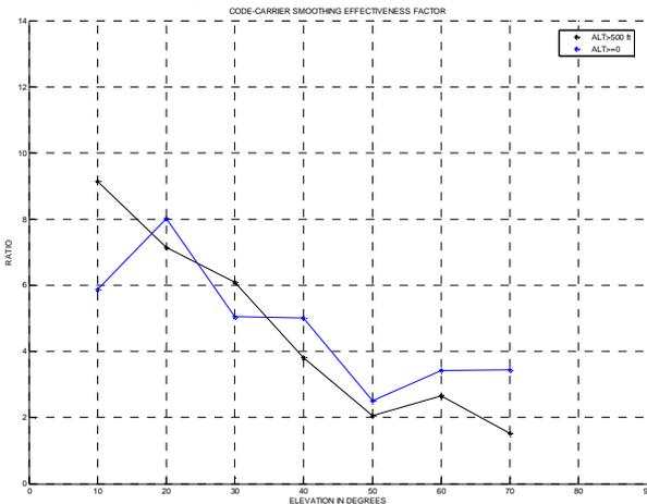
**Figure 17:** Code-carrier smoothing effectiveness factor (GPS L1 C/A, BW<sub>2</sub>=2 MHz, C<sub>S</sub>=1 chip, 500 approaches per sat elevation, A340).
