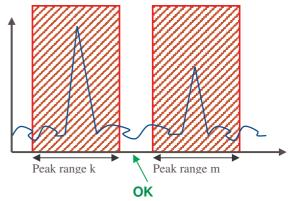
Fig 6 Collisions between satellites having close code delays
