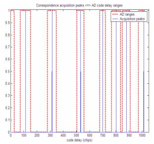
Fig 9: The relationship between the acquisition peaks and the different AD ranges for the first group of 7 satellites
