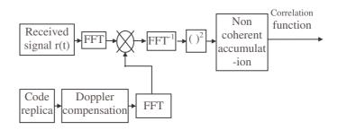
Fig 1 Classical GPS acquisition scheme
