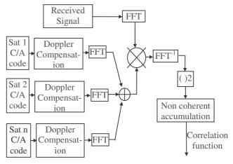
Fig 3 SOR algorithm principle
