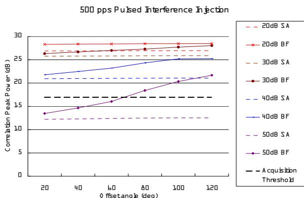
**Figure 10. 500 pps Pulsed Interference Rejection Performance**
