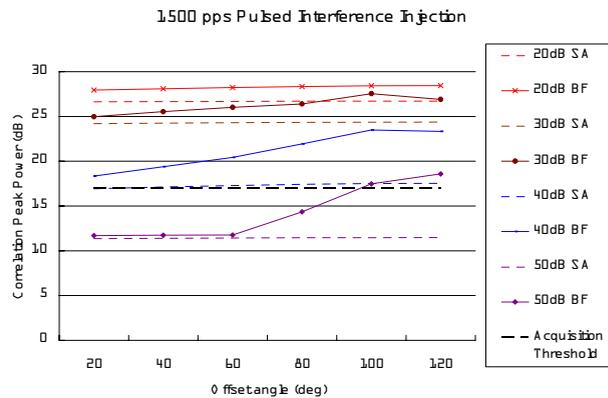
**Figure 11. 1500 pps Pulsed Interference Rejection Performance**
