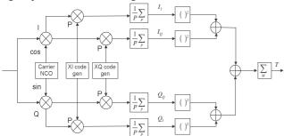
Figure 2: L5 acquisition structure.
