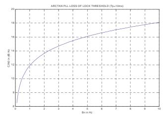
Figure 13: Arctan PLL loss of lock threshold (composite data+pilot L5 signal C/N<sub>0</sub>) as a function of PLL equivalent noise bandwidth.
