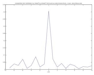
Figure 5: Cross-correlation between 1ms correlator outputs and local NH20 (residual Doppler=25 Hz).
