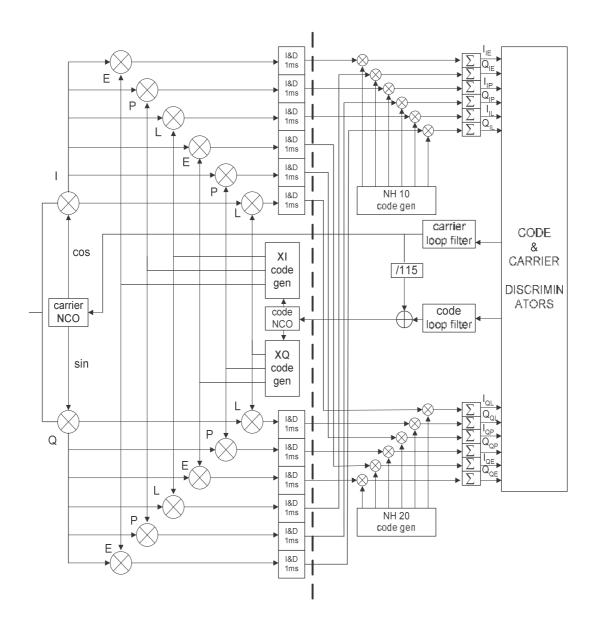
Figure 1: Proposed L5 tracking loops structure.
