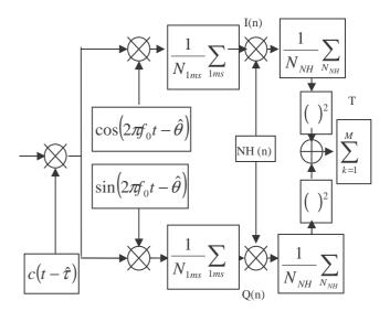
Figure 3: NH acquisition structure.
