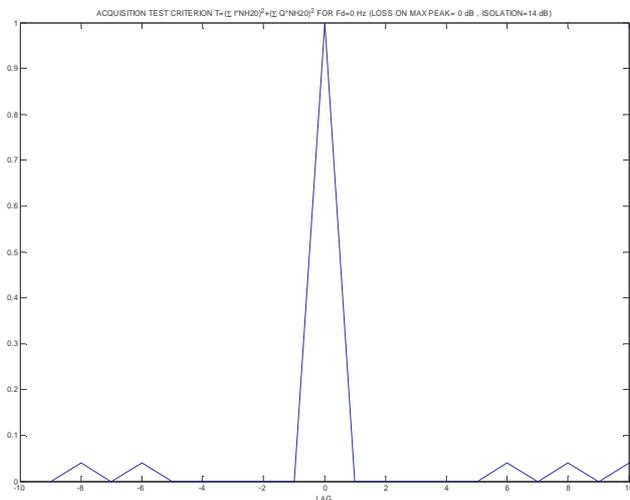
Figure 4: Cross-correlation between 1ms correlator outputs and local NH20 (residual Doppler=0 Hz).
