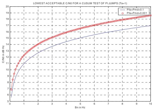
Figure 12: Lowest acceptable data or pilot channel  $C/N_0$  as a function of loop noise bandwidth to test for pi jumps in the classical arctan discriminator when  $T_p=10$  ms.
