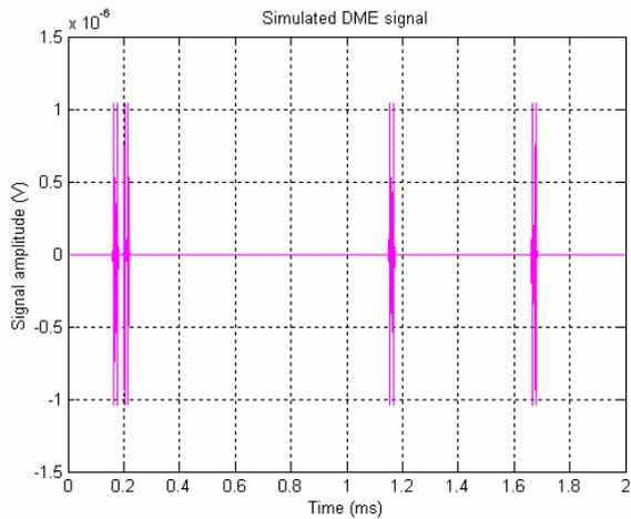
Figure 10 Simulated DME signal over 2 ms
