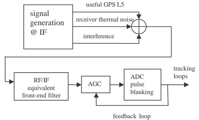
Figure 1 L5 receiver simulator diagram
