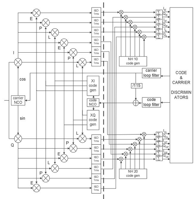
Figure 6 L5 receiver simulator tracking loops diagram
