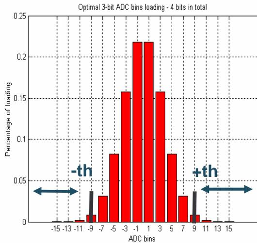
Figure 4 Optimal 3-bit loading using a 4-bit ADC
