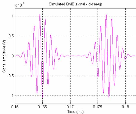
Figure 11 Close-up on the first generated pulse pair
