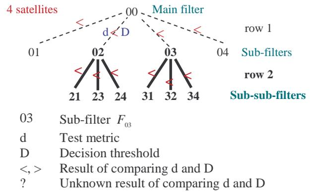
Figure 4. Test metrics vs decision threshold: no-failure case.
