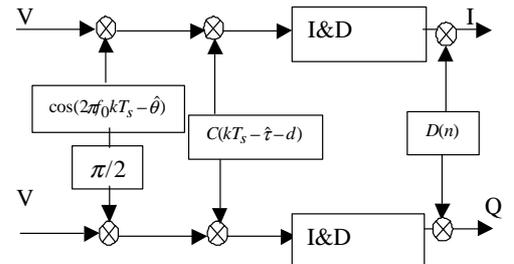
Figure 3: Architecture of one correlator output.
