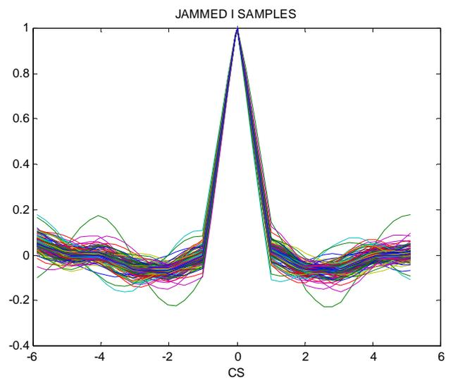
Figure 8: Observed correlation peaks when jammer is on.
