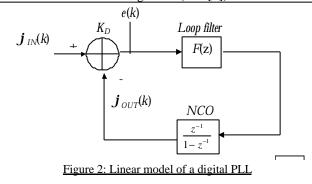
linear model of a DLL (see [1]) is the same as for the PLL where the carrier phase is substituted by the code phase. The local code generator and the local carrier generator are both modeled by a digital integrator. The gain KD is the product of the discriminator gain with the Numerically Controlled Oscillator (NCO) gain. The transfer function F(z) of the loop filter of an  $N^{th}$  order loop is modeled as
