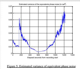
That's the reason why we choose to implement a second order FAB PLL. We know that for second order loops, the bias on the phase measurements is proportional with the LOS acceleration. It means that the noise will be low powered when we need to open the loop bandwidth to track high acceleration and that acceleration will be low when the noise is powerful. This results on a good
