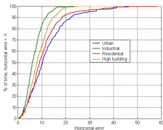
**Figure 14: Percentage of time function of position error for different environments**
