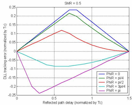
**Figure 4: Multipath tracking errors function of PhiR**
