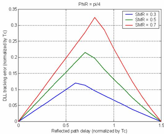
**Figure 3: Multipath tracking errors function of SMR**
