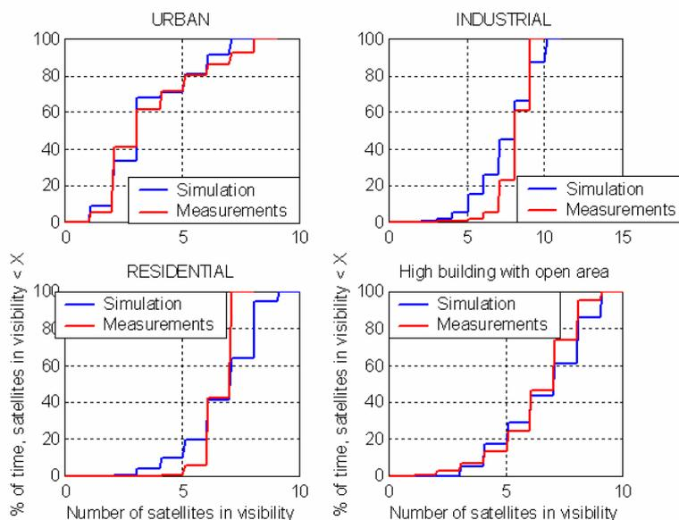
**Figure 9: Comparison between measurements and simulation results**
