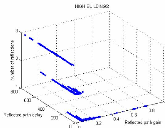
**Figure 13: Path characteristics in medium with high buildings**
