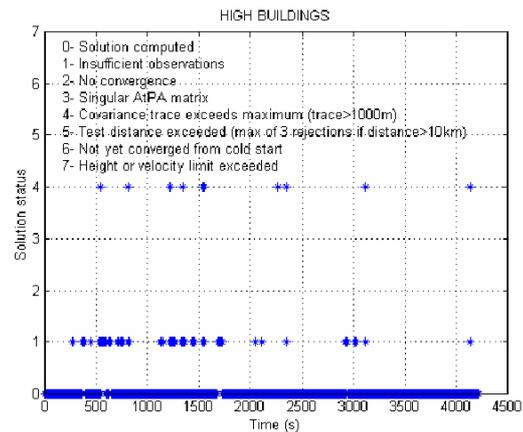
Figure 8 : Solution status in medium with high buildings
