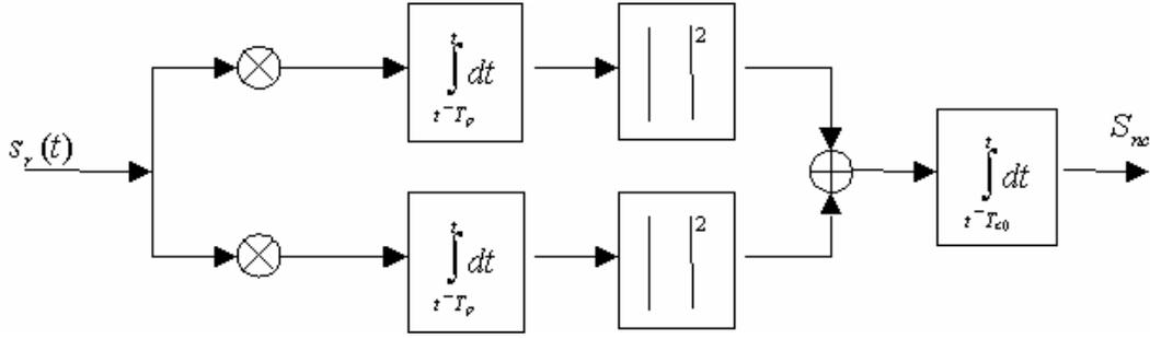
**Figure 2: Non coherent delay lock loop phase detector**
