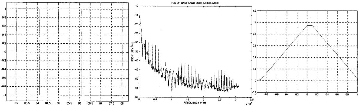
Figure 2: Model A Evil Waveform:  $\Delta=0.1 T_c$
