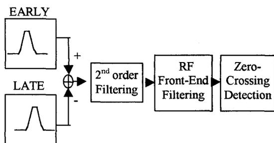
Figure 6: Architecture of simplified GPS receiver simulator.
