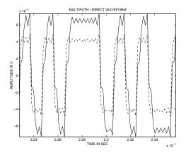
Figure 2: Comparison between the received and Figure 3: Comparison between the received waveform with multipath (solid) and the received waveform without multipath (dashed). The only obstacle is a reflecting wet soil for a receiving antenna placed 50 m above the plate.
