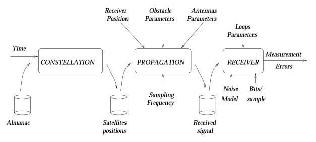
Figure 1: Data flow for the simulator.
