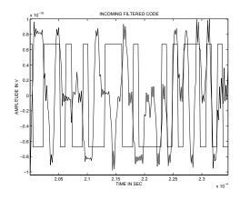
the transmitted waveform when the only obstacle is a reflecting metallic plate for a receiving antenna placed 50 m above the plate.
