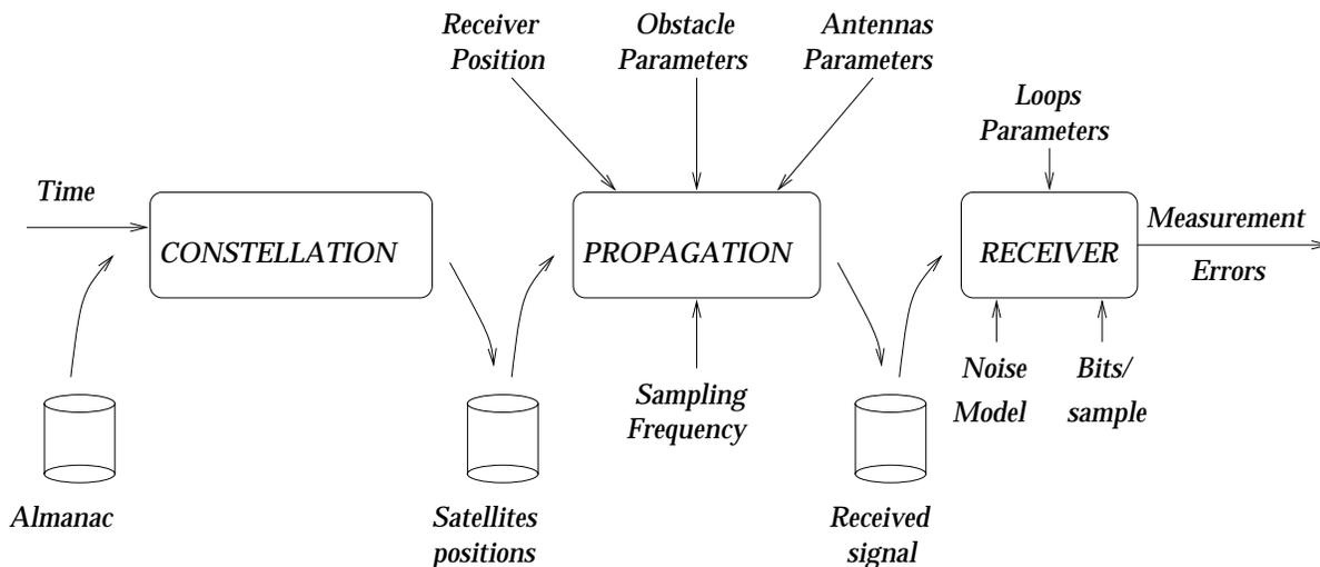
Figure 1: *Data flow for the simulator.*
