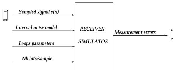
Figure 3: *Data flow for the receiver simulator.*
