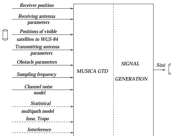
Figure 2: *Data flow for the propagation simulator.*
