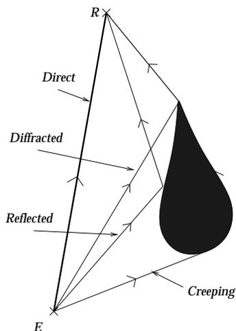
Figure 8: Illustration of the different considered rays.
