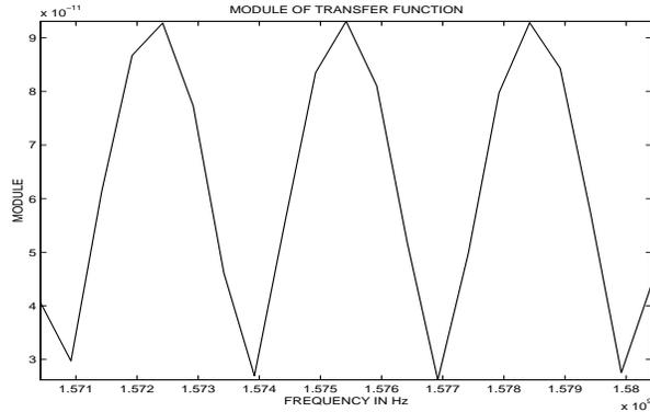
Figure 6: Example of variation of the transfer function of the GPS propagation channel  $\pm 10$  MHz around L1. This function was obtained from the simulation of a signal reflected by wet soil for a receiving antenna located 50 m above the ground.
