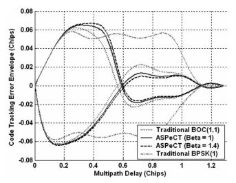
Fig. 14. Code tracking multipath envelope for traditional sine-BOC(1,1), traditional BPSK(1), and ASPeCT ( $\beta$  = 1 and  $\beta$  = 1.4) for an early-late spacing of 0.2 chips, and a 6 MHz front-end filter (double-sided).
