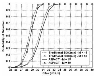
Fig. 15. Probability of detection for proposed civil Galileo L1 signal assuming coherent integration time of 4 ms, noncoherent summations of 15 and 50, no code delay error, and probability of false alarm of  $10^{-3}$ .
