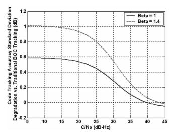
Fig. 13. Code tracking error standard deviation degradation for ASPeCT and traditional sine-BOC(n,n) versus  $C/N_0$  for  $\beta=1$  and  $\beta=1.4$  for an early-late spacing of 0.2 chips and a coherent integration time of 1 ms.
