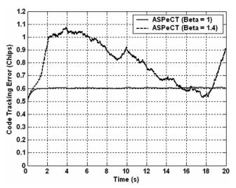
Fig. 11. Code delay error for a sine-BOC(1,1) signal tracking starting with an initial code delay error of -0.5 chips (2 Hz DLL), an integration time of 1 ms, and for a  $C/N_0$  of 50 dB-Hz for ASPeCT ( $\beta = 1$  and  $\beta = 1.4$ ).
