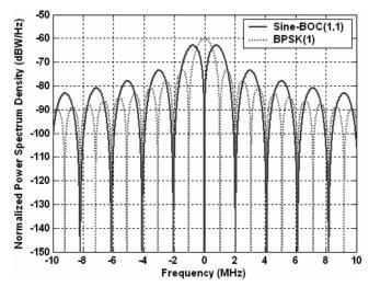
Fig. 1. Normalized sine-BOC(1,1) and BPSK(1) power spectrum densities.
