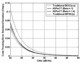
Fig. 12. Code tracking error standard deviation versus the  $C/N_0$  for the traditional sine-BOC(n,n) tracking and ASPeCT ( $\beta=1$  and  $\beta=1.4$ ) with an early-late spacing of 0.2 chips and a coherent integration time of 1 ms.
