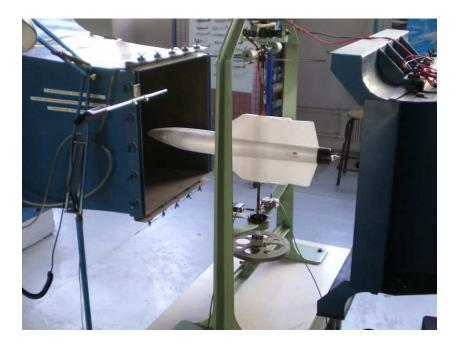
Figure 1.2: wind tunnel experiment for propulsion
