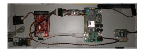
Figure 3.1: Breadboard prototype of the new flight computer.
