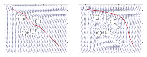
Fig. 3. Trajectories computed with a Neumann harmonic navigation field and a biharmonic navigation field. Starting point : bottom right, destination point : top left.
