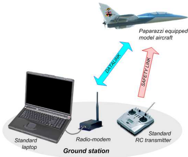
Figure 1: Paparazzi Aircraft Components
