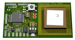
Fig. 4. The *tiny* controller board includes a GPS receiver and antenna
