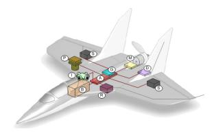
Fig. 5. The Paparazzi airborne system components: (A)utopilot Control Board, (B)attery, (D)atalink Radio-Modem & Antenna, (G)PS Receiver, (I)R Sensors Board, (M)otor & Controller, (R)C Receiver & Antenna, (S)ervos, (P)ayload = Camera & Video Transmitter
