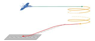
Fig. 7. The landing circuit pattern is composed of three steps which are join, descend and glide.
