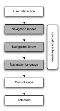
Fig. 6. The navigation subsystem is composed of three layers, the link between the interactive command of the system and the low level control loops managing the actuators.
