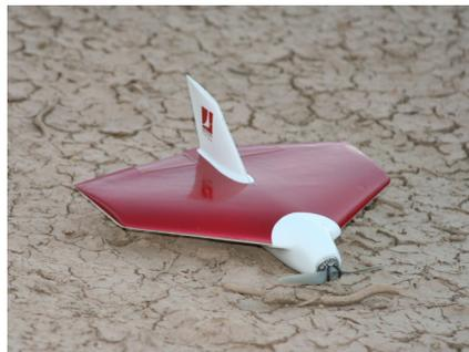
Fig. 1. The 30cm span, 300g Slayer from Miraterre Flight Systems.
