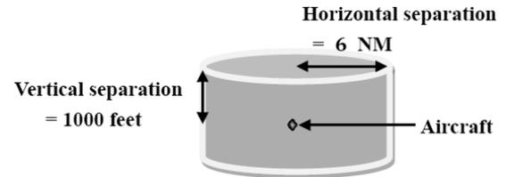
Figure 2: Aircraft protection zone cylinder in 3D
