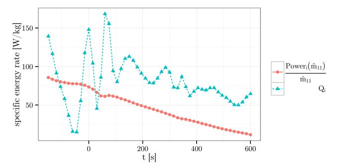
Figure 1: This figure portrays the computed specific energy rate  $\frac{Power_i(\hat{m}_{11})}{\hat{m}_{11}}$  and the observed specific energy rate  $Q_i$ . In this figure,  $\hat{m}_{11}$  was estimated with the least squares method. The largest error on the predicted altitude at the time t=600s is obtained with this trajectory.
