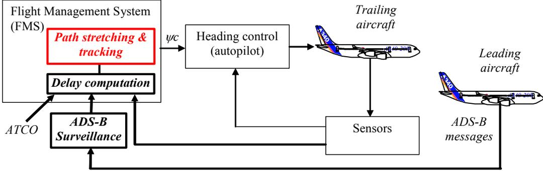
Figure 1: Path stretching & tracking feedback loop
