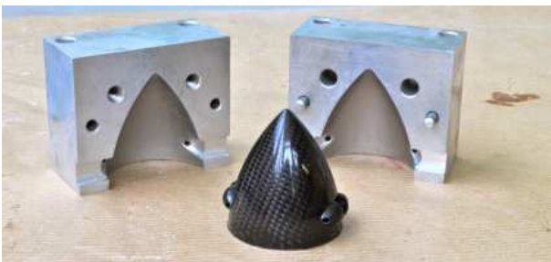
Figure 20: The cone and its molds
