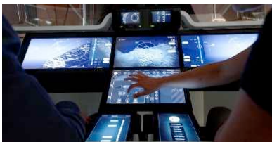
Figure 2 : Avionic 2020 tactile screens.
