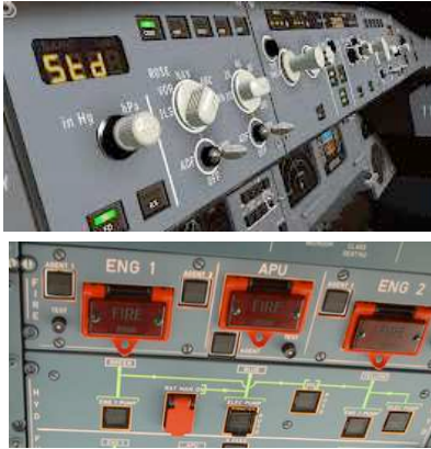
Figure 3 : (top) Airbus FCU physical buttons (Flight Control Unit); (bottom) overhead panel: guarded buttons.
