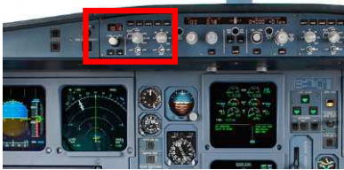
Figure 1. a) Navigation and flight displays in the cockpit of a TB20; b) buttons of the EFIS (Electronic Flight System) control panel that control the display mode of the navigation display (ND) (2 nd from the left).
