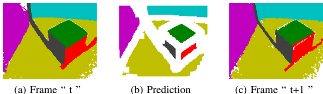
Fig. 9: Planes Tracking and Matching across a sequence of frames. By eroding frame “ t ”, planes are predicted in frame “ t+1 ”
