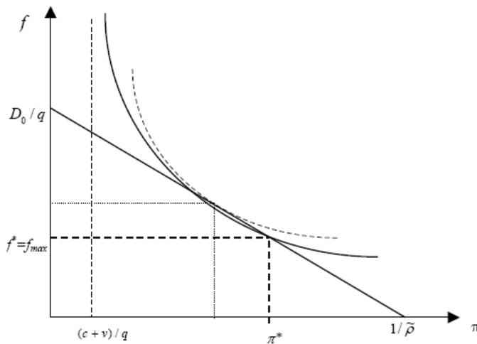
**Figure 3:** Optimization of airline profit with an active fleet constraint at full capacity
