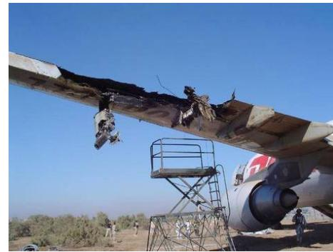
Fig. 1 The damaged left wing after landing
