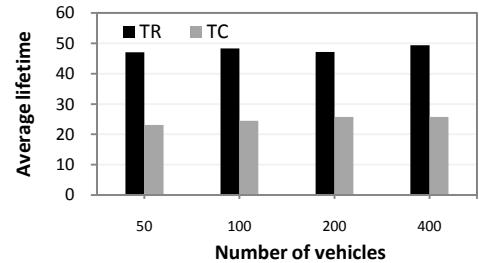
Fig. 6. Average connections lifetime vs. Nodes density
