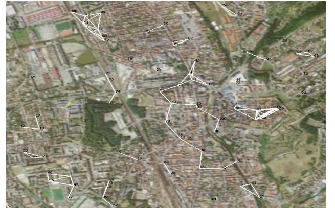
Fig. 1. Initial connection graph for 100 vehicles distributed in an area of 2500m\*2500m.
