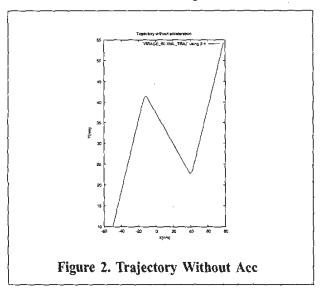
A 30 kts wind coming from the north has also been included in the simulation. After simulation, we have 30 estimated trajectories and one reference trajectory. For each time step, the differences between the estimates and the reference are computed. Wind errors in magnitude  $\varepsilon_{\theta}(k)$  and direction  $\varepsilon_{\parallel \underline{w} \parallel}(k)$  are then computed. The power of those error are evaluated:
